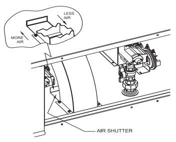
Figure 54 – Adjusting Air Shutter 990,000 - 2,070,000 Btu/hr Models
